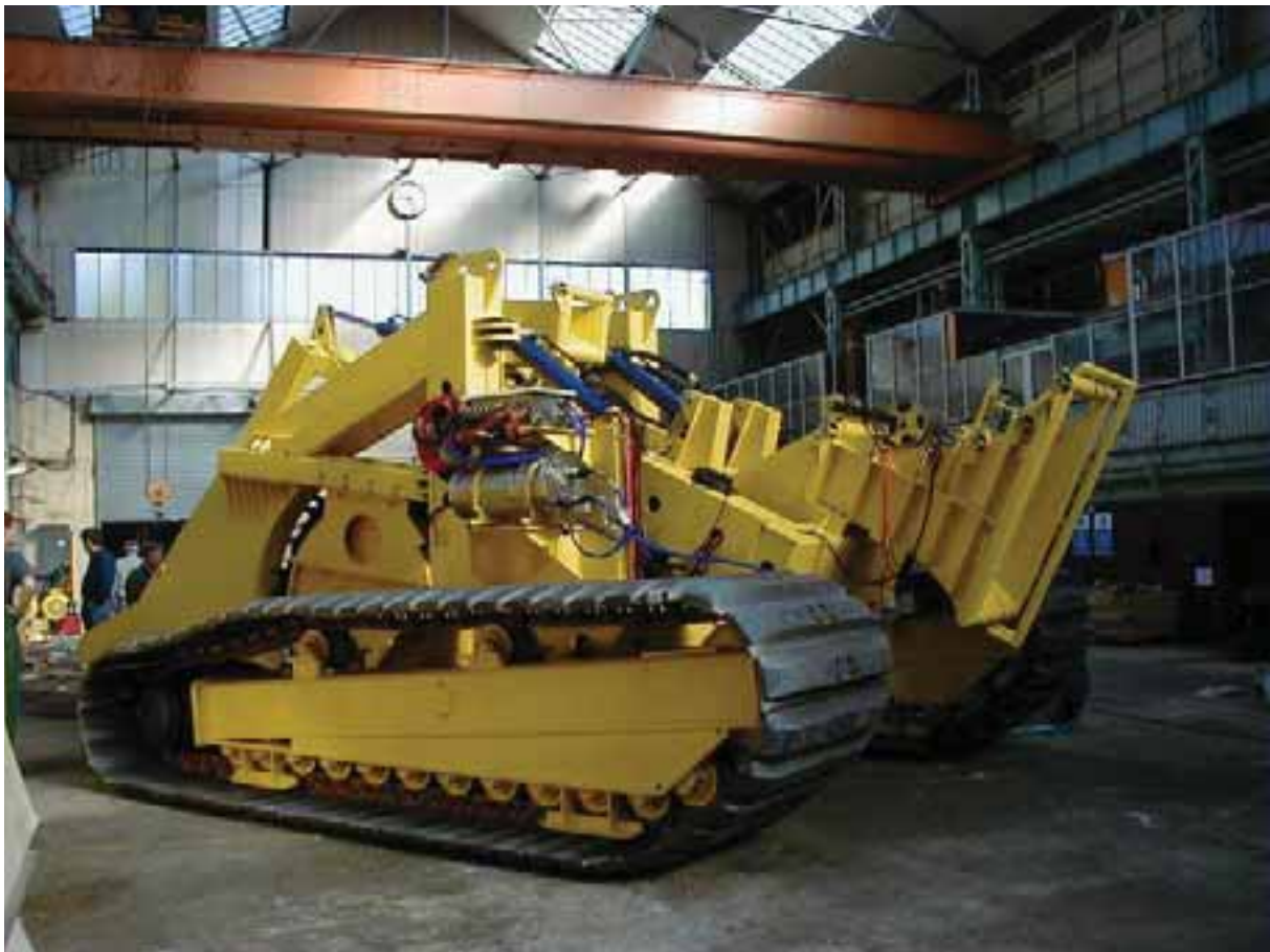
Figure 3.18: Shallow Water Tracked Cable Burial Machine Fitted with a Rock Wheel Cutter
